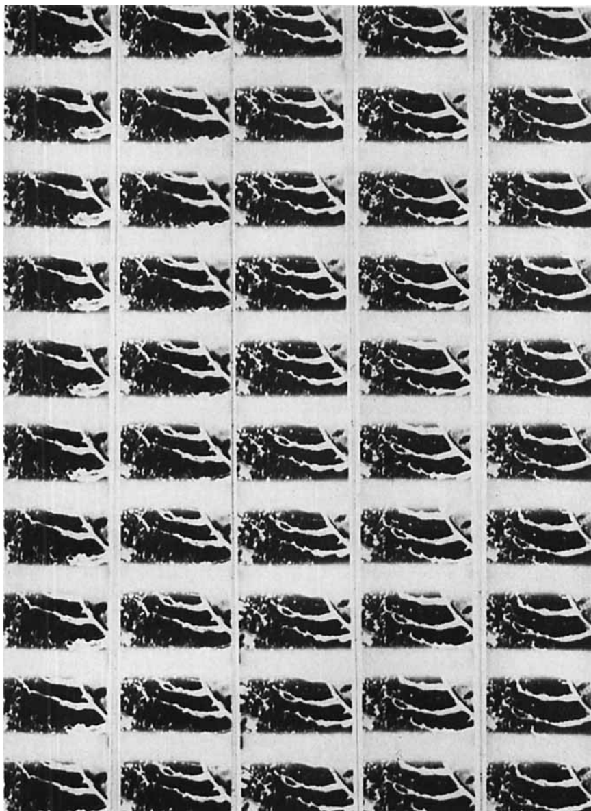
FIG. 18. HIGH-SPEED MOTION PICTURE FRAMES SHOWING COARSE LIGAMENTS FORMED AT LOW DISK SPEED; N = 640 REV./MIN., w = 30 LB./MIN.
